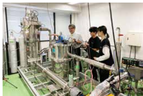
極低温流体輸送試験装置での実験 Experimental study on cryogenic fluid transport test equipment
