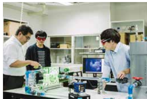
PIV を用いたエネルギー機器内流れ計測 Study for internal flow field of energy device using PIV
