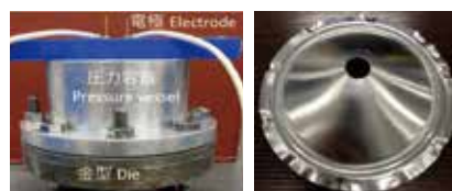
高電圧放電による水中衝撃波を用いた金属板の高速成形 High-Strain-Rate Metal Forming Using an Underwater Shock Wave by High Voltage Discharge
