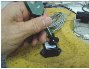
Fig.1 Measuring acceleration by 128Hz tuning fork.
