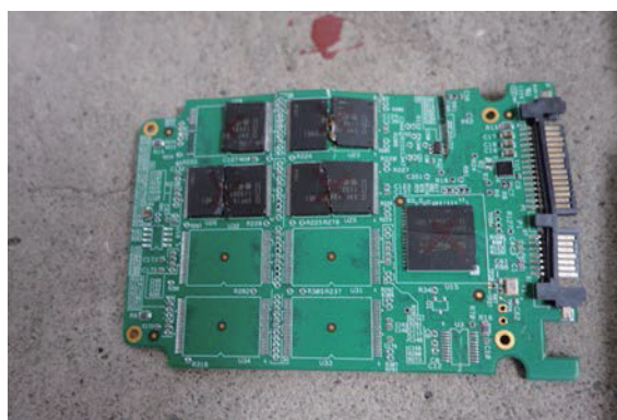
図7 SSD内のチップを破壊 (Fig. 7 Destruction of the chip inside the SSD)
