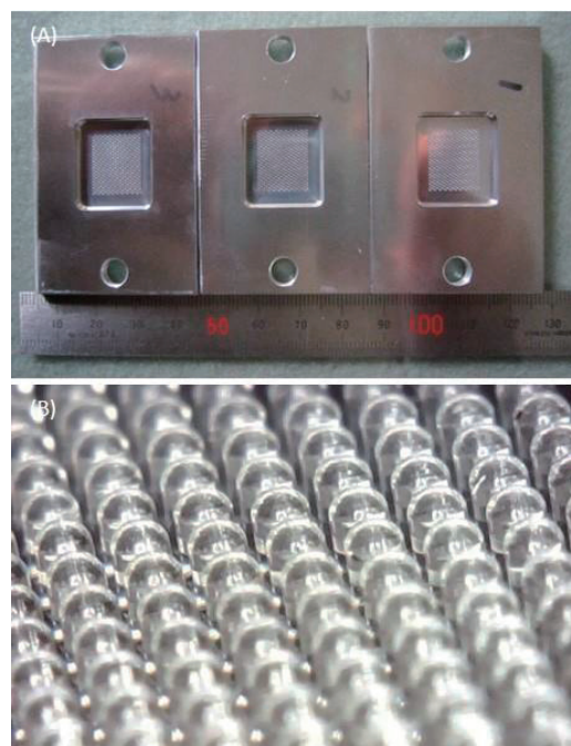
Fig.7 Top view of primary mold (Aluminum alloy) (A) and surface of the secondary mold (PDMS) (B).
